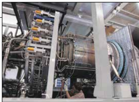
FIGURE 2. Gas turbines typically have a defined operating speed range. When used in a machinery train (with a generator, compressor or pump train), a well-designed gear unit is used to match the speed of the turbine shaft to the driven equipment
