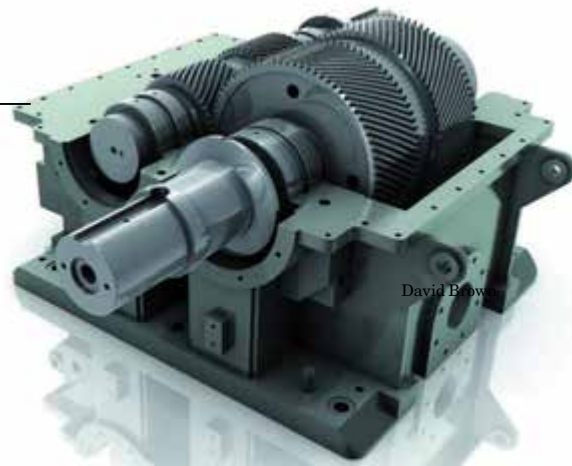
FIGURE 1. In this conventional, double-helical gear unit (with a welded-steel casing), double-helical gears are used to minimize the axial load (that is, the load in the direction of the shaft). The complex casing was fabricated by welding
