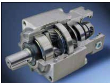
FIGURE 3. In this planetary gear unit, the transmitted power is divided over several teeth. Planetary gear units are smaller, more compact and cheaper than their conventional counterparts
