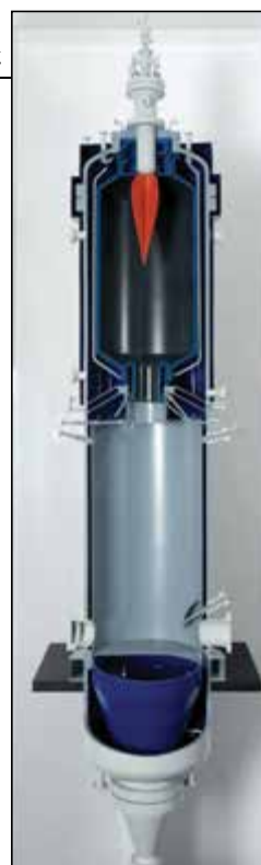
FIGURE 1. The Siemens coal gasifiers, which are 18-m long, 3-m I.D. and weigh 220 metric tons (m.t.), are among the world's largest and most powerful. They are capable of gasifying up to 2,000 m.t./d of coal. The photo shows a cross section through the reactor of a coal gasifier
